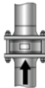
Vertical pipe with flow UP
