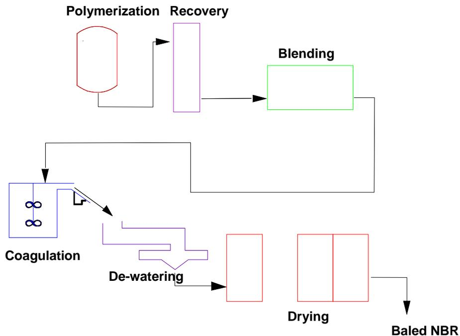
**Figure 2: NBR Manufacturing Process**
